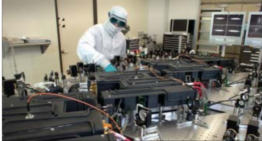
A technician at Northrop Grumman Space Technology checks diagnostic instruments used to monitor IR laser beams fired by a laboratory demonstrator for the JHPSSL program.
