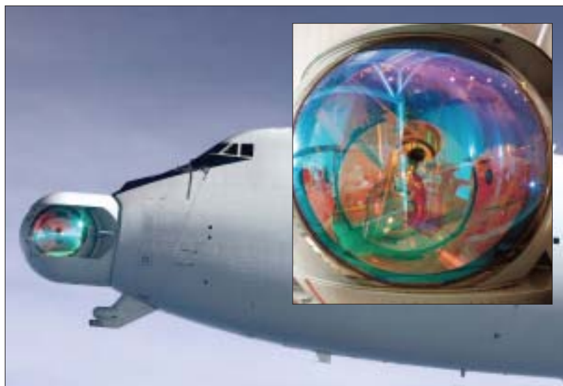
The ABL will reside in the nose of a modified Boeing 747-400.
